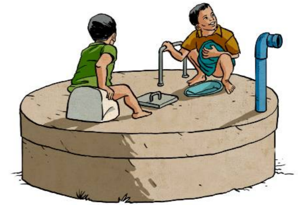
The Potty Hub consists of two pans, a squat pan and a potty, built directly onto a pit.
