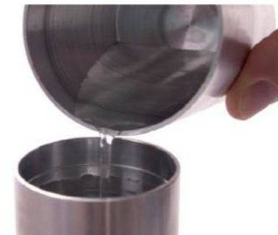
Figure 8. Pour water sample up to 100ml line
