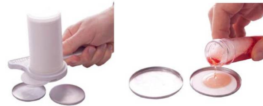
Figure 6. Dispense a growth pad into a sterile petri dish and saturate with MLSB.
