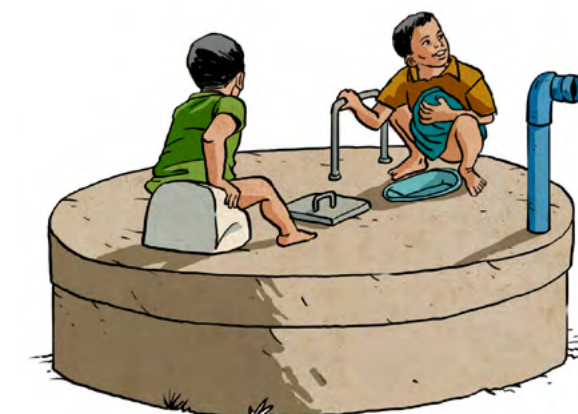
The Potty Hub consists of two pans, a squat pan and a potty, built directly onto a pit.
